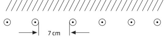
Correction factor (f<sub>2</sub>) for cables laid underground as shown below.
