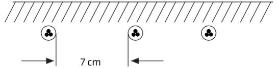
Correction factor (f<sub>2</sub>) for cables laid underground as shown below.
