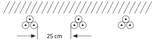
Correction factor (f<sub>2</sub>) for cables laid underground as shown below.
